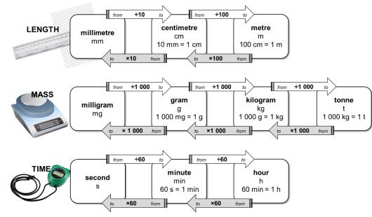
For example, to convert a length in millimetres into units of centimetres, divide by 10, eg 10 mm = 1 cm.
